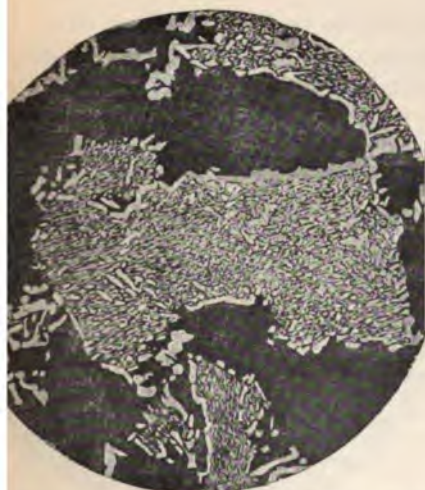
10.—SOFT-GRADE CEMENTED BAR—LAYER BETWEEN CENTER AND OUTSIDE OF BAR— CARBON 0.5%. Magnified 125 diameters.
